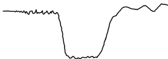
Fig. 1. The typical oscillogram of the output pulse of a klystron modulator.
